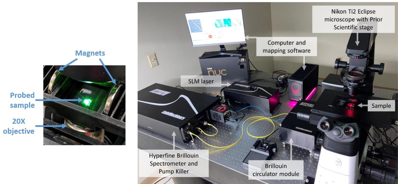
**Figure 1. Left:** Picture of sample mounted between two permanent magnets in Brillouin microscope. **Right:** Experimental setup for Brillouin spectroscopy. The single longitudinal mode laser, the Brillouin circulator module, the HyperFine spectrometer, and the Pump killer are fiber coupled. The Brillouin circulator module is coupled to the Nikon microscope via the left camera port.
