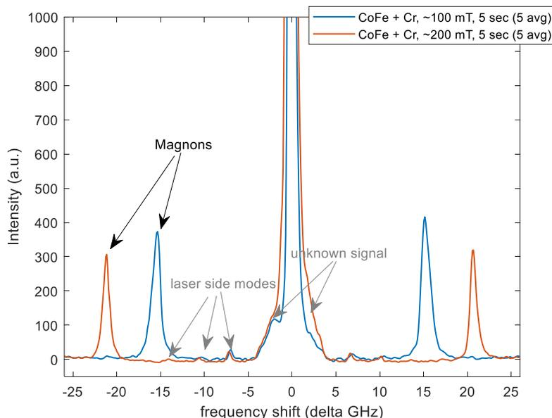
**Figure 2.** Spin wave Brillouin spectra of the CoFe sample for two different magnetic fields. Experimental conditions: backscattered geometry, sample at normal incidence,  $\sim 20$  mW at the sample, 5 sec exposure averaged 5 times, 20X objective.
