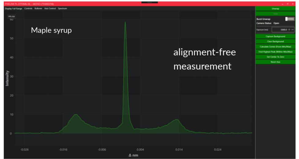
Ultra-high throughput: high signal-to-noise Brillouin signal in milliseconds is possible; Large spectral range in a single snapshot (>2 THz): can measure hard materials and even ultra-low frequency Raman spectra;
