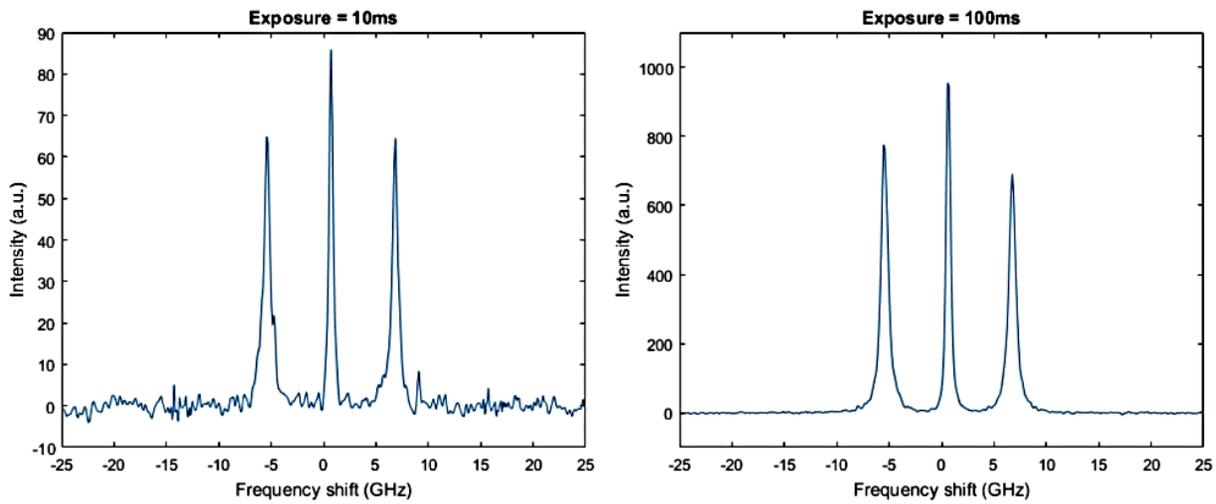
**Figure 8: Example of Brillouin signals (from Table 1).** For reference only (intensities will vary depending on the config file settings, so SBR measurements are better references). 50 mW of laser power at the sample. 660 nm, 20X objective.
