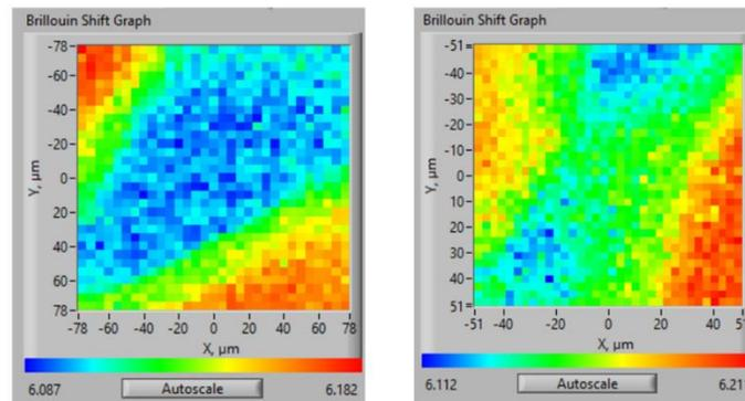
**Figure 4: 2D maps presenting the Brillouin frequency shifts of non-uniform hydrogels.** The colormap scale is given in GHz.
