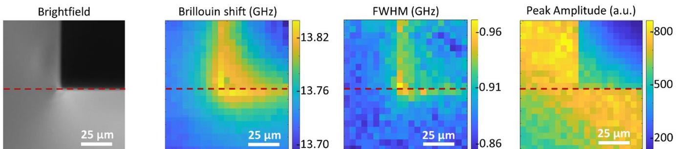
**Figure 3: Sharp silica glass corner encapsulated in epoxy glue.** The brightfield image is presented on the left, followed by the Brillouin shifts, FWHM, and peak amplitude maps. Red dashed lines have been superimposed to each image along the glass cube boundaries to facilitate image comparison.
