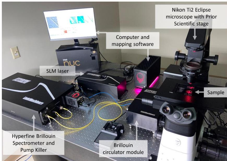
**Figure 2: Experimental setup for Brillouin mapping.** The single longitudinal mode laser, the Brillouin circulator module, the Hyperfine spectrometer, and the Pump killer are fiber coupled. The Brillouin circulator module is coupled to the Nikon microscope via the left camera port.
